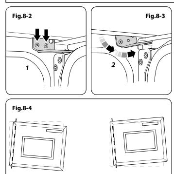
Effect of hinge adjustment - exagerrated for clarity
